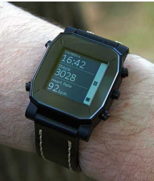
The Agent Smart Watch, prototyped using an Atmel SAM7X-powered Netduino, offers two-way communication to smartphones, wireless charging, and long battery life.
